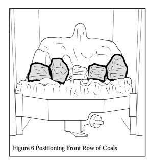
Install the 14 loose coals as follows. Begin the coal build by placing a single coal in the centre of the front coal, ensuring that it bridges across to the matrix as shown in figure 5.
