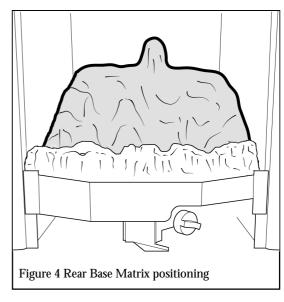
Place the rear base coal matrix in the burner compartment behind the front coal. It should rest on the ledge at the back of the burner compartment. (See Figure 4).
