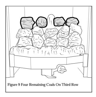
Place the remaining four coals behind the second row of coals, two each side of the centre coal shape formed within the matrix. (Fig. 9)
