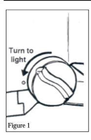
This fire is controlled by a 4 position gas tap mounted on the front leg of the appliance (see Fig 1). In addition to the OFF position there is a pilot light and 2 heat control settings.
