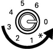
THERMOSTAT KNOB To shut down the boiler turn anti-clockwise
