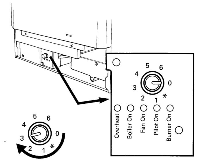
Your boiler is fitted with an additional safety device which shuts down the appliance should the system overheat. If the pilot is extinguished for no apparent reason and cannot be re-ignited, this overheat cut-off device may have operated.
