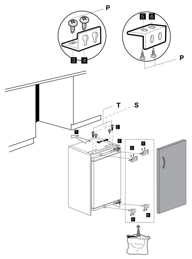
**Note:** Installation step for 2, screws for connecting top plastic rpart should not be screwed very **hard** because of moving the plastic part easily left or right side.
