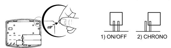
1) ON/OFF - boiler switches ON when below set temperature and OFF when above..
