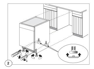
4. If necessary, pads are supplied for the rear feet to make sliding the appliance in and out of the recess easier. To fit the pads, press them onto the rear feet.
