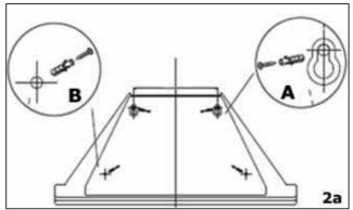
**2a)** The support screw holes are indicated by figure **A** in this drawing and the anchoring screw holes are indicated by figure **B**.
