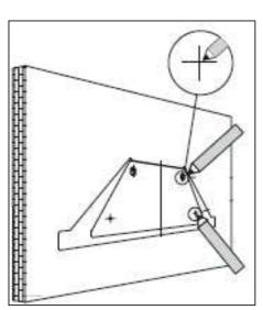
2) Position the extractor against the wall that you are intending to install it on and mark the position of the support holes that are to be drilled (as shown in the figure below).
