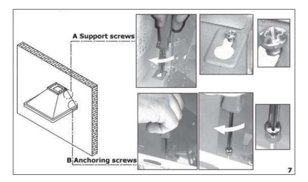
**7)** Fully tighten the support screws **(A)** and then screw the anchoring screws **(B)** through the relevant holes in the extractor. Fully tighten the anchoring screws into the wall.
