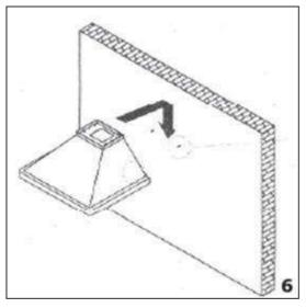
**6)** Hang the extractor onto the support screws.
