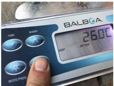
Set To sleep between clients, when in sleep mode ALWAYS reset temperature to minimum temperature which is 26, this will have the tub run at around 15.
