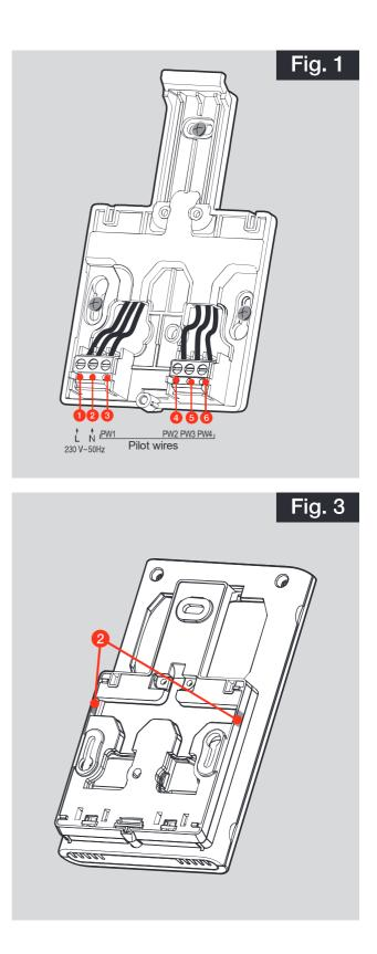
Partitions (2) that can be removed by pliers are provided for passing the connection wires if required. - See Fig.3 Turn the control dial to  $\uparrow$  and press
