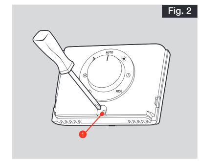
Secure the base using three screws or fit onto a flush-mounted box (distance between centres 60mm).
