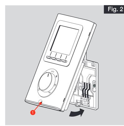
Fit the programmer onto the tab of the base and secure it with the clamp screw **1**
