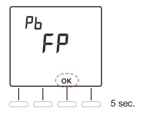
Check the connection of the pilot wires to the heaters and resolve any connection problems. When the check has been carried out, test the pilot wire again by pressing OK for 5 seconds (time taken for the test to complete: approx. (1 minute 30 sec).
