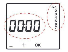
Reset the time. Turn the control dial to (). The days flash. Press + or - to make your choice, **OK** to confirm it and go to the next setting.
