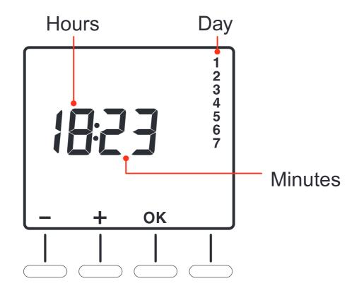
Repeat the operation to set the hours and minutes. Turn the control dial to exit the setting mode.
