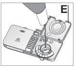
The rinse aid is specially formulated to be used in the dishwashers for the prevention of watermarks and scale on dishes and to increase the efficiency of the washing and drying processes. Therefore, make sure that there is adequate amount of rinse aid in the rinse aid dispenser of your machine.
