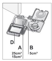
container (A) up to 25cm3 level. If the dishwasher is not quite full and the dishes are only slightly soiled, fill the main container (A) only up to 15cm<sup>3</sup> level.
