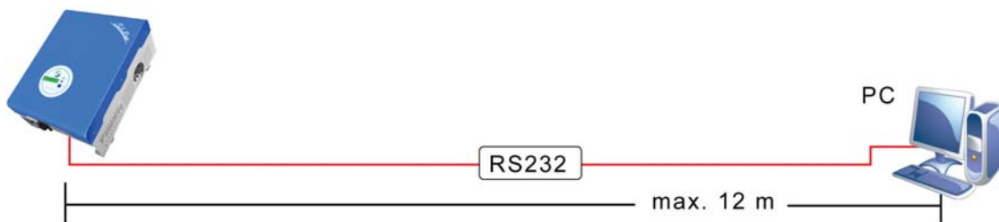
Figure 21 RS232 Communication Diagram
