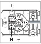
1. Open the terminal board by inserting a screwdriver into the side tabs of the cover. Use the screwdriver as a lever by pushing it down to open the cover (see diagram). 2. Install the power supply cable by loosening the cable clamp screw and the three wire contact screws L-N-Connect the wires to the corresponding terminals: the Blue wire to the terminal marked (N), the Brown wire to the terminal marked (L) and the Yellow/Green wire to the terminal
