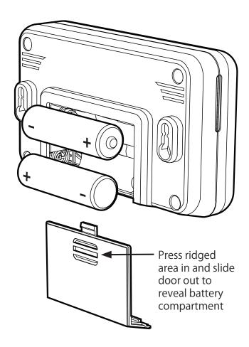
Under normal operating conditions, the batteries should last for at least 12 months.
