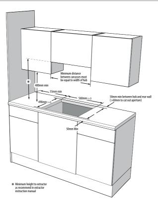
No shelf or overhang of combustible material should be closer than 650mm directly above the hob.
