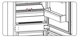
When the humidity controler in the closed position, it allows fresh fruit and vegetables to be stored longer.
