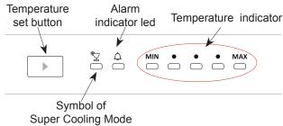
This button allows setting temperature of the fridge. In order to set values for fridge partition, press this button. Use this button also to activate Super Cooling mode.
